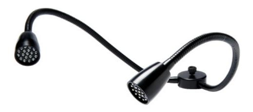
Spot light with 19 + 19 LEDs on two semi-flexible arms (goose-neck) provides exceptionally bright and homogenous illumination. The product is designed for assembly on Optilia Stands with  $\phi$ =3/4" (19.05mm) vertical rods. Illumination intensity of the spots can be adjusted by the included control unit. Colour filters (optional) can be assembled on front of the spots if required.
